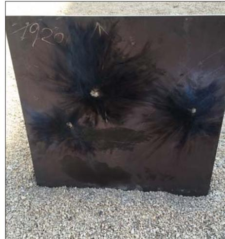
Actual bullet test for armour steel-B7 protection grade
